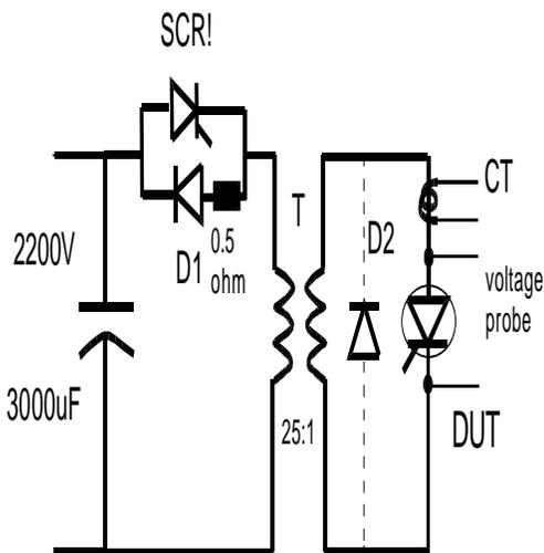
Fig.3 Type of laboratory circuit used to verify or establish ratings for  $I_{TSM}$  and pulse power
