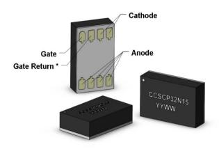
\*The **Gate Return** pad provides a dedicated connection directly to the cathode of the semiconductor die. This connection consists of a single 0.010" aluminum bond wire.
