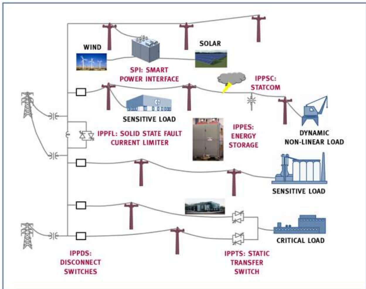
Figure 2. Macroprocessor applications in medium-voltage class distribution systems
