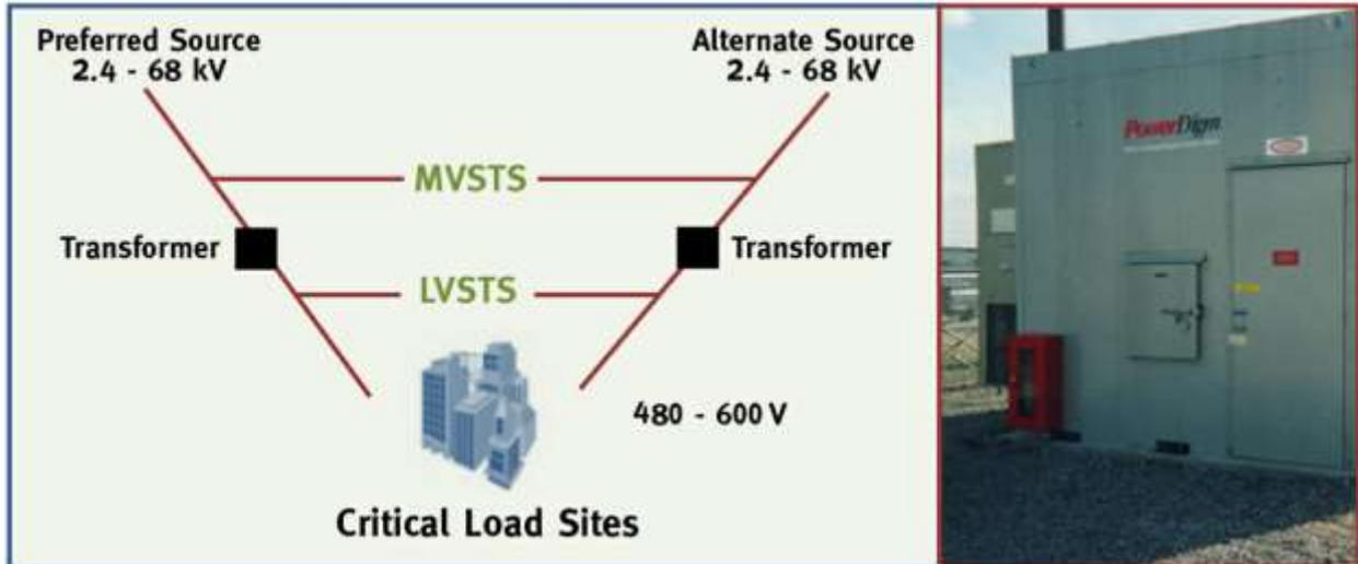
**Figure 3. SPCO's static transfer switch (STS) rapidly switches utility service to the critical load from a source/feeder affected by an interruption to an alternate source.**
