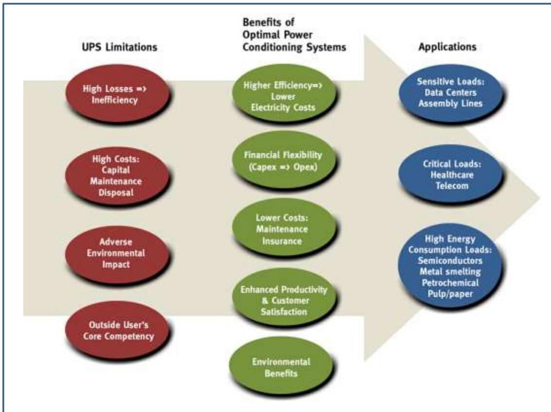
Figure 1. UPS limitations, benefits of optimal power conditioning systems, and applications
