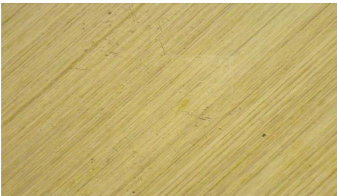
Figure 1. illustrates the typical results of the optical inspection of the samples. Striation due to back-grinding and surface scratching was observed on all samples.
