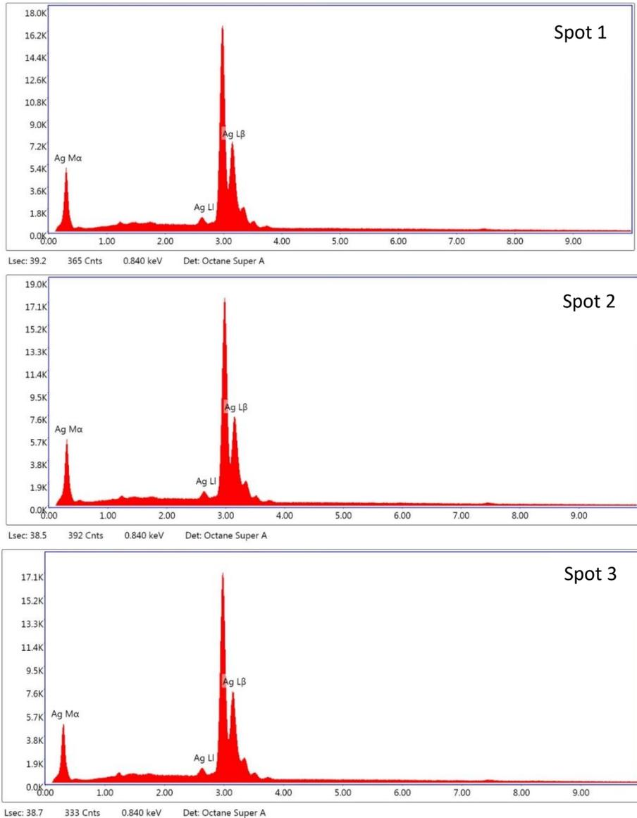
Figure 6: EDS Results Illustrating No Nitrogen Peaks (DMEA)
