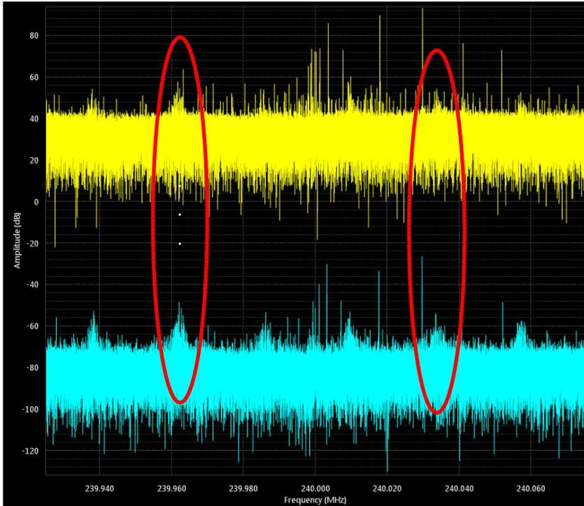
Figure 2: Typical EM Analysis Result: Comparative analysis of the 240 MHz Bandwidth. Known Good Sample (Yellow) and modified (Back Grind) Sample (Blue)
